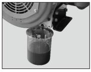
Open the lock over the front cover, screw the oil cap off as shown in the photo, pour the oil until reaching the limit of the oil gauge. Finally, screw back the cylinder head stud.
