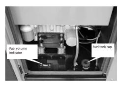
Open the left door, check the fuel volume indicator. If the fuel level is low, unscrew the tank cap, fill the fuel through the fuel filter. After filling fuel, screw back the tank cap.
