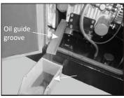
Open the lid on the top of generator, unscrew the oil cap then fill the oil until reaching the limit of the oil gauge. Finally, screw back the cylinder head stud.
